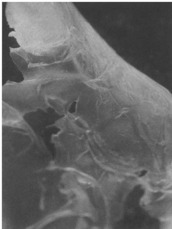
Fig. 4. Microscopic picture of a cast film of EuSMe 110 after a period of 60 min at pH 8 (magnification, 10 \times ).
